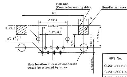
Unit:mm No. of Pin HRS No. С Part No. Α CL231-3006-8 9.96 6.35 23.96 3110-6S CL231-3001-4 8 3110-8S 12.5 8.39 26.5 CL231-3008-3 12 3110-12S 17.58 13.97 31.58
