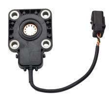
The 8360 Series is BEI Sensors' latest addition to the company's line-up of robust, reliable, and highly accurate non-contacting position sensors. The 8360's low profile and throughhole design make it desirable for applications like steering wheel and boom angle, where space is limited and the sensor must mount around a shaft. The sensor's dual analog output is capable of resolving 360 degrees of motion with high accuracy and 12 bit resolution.
