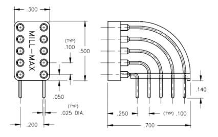
**Description:** DIP Display Socket 10 Position Vertical Mount DIP Through Hole Plating Code:
