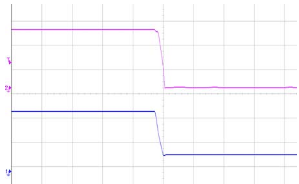
Figure 7 Output voltage shut down by power off, (50ms/div), see Figure 10 for test configuration; CH2-output voltage (5V/div); CH1-input voltage (20V/div)
