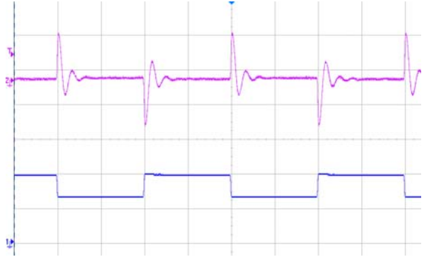
Figure 5 Dynamic response for 25% load step (50% ~ 75% ~ 50%) and 1A/μs slew rate, (2ms/div), see Figure 10 for test configuration; CH2-output voltage (200mV/div); CH1-output current (10A/div)
