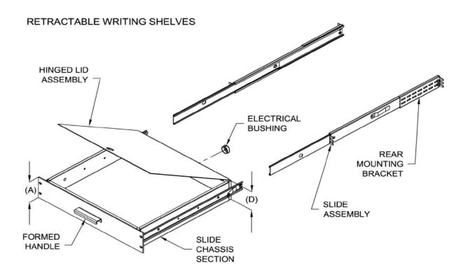
Slide assemblies with rear mounting brackets and assembly hardware as follows:
