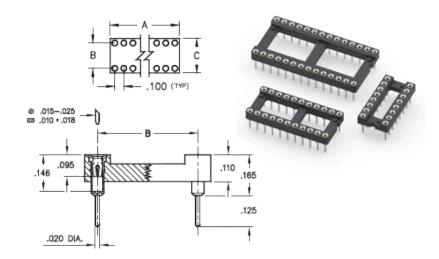
Description: DIP Dual In Line Socket Standard Solder Tail Open Frame Through Hole Plating Code: Shell Plating: 10 μ" Gold over 100 μ" Nickel Inner Contact Plating: 30 μ" Gold over 50 μ" Nickel Packaging: Packaged in Tubes
