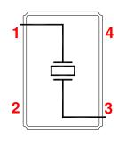
Pad 2 and Pad 4 are common and connected to the metal cover. They are not connected to the crystal.
