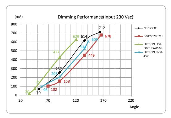
Triac dimming performance is typical as with other models, for specific details on other model performance, please see the Aimtec Triac Dimming Application note at <a href="https://www.aimtec.com">www.aimtec.com</a>
