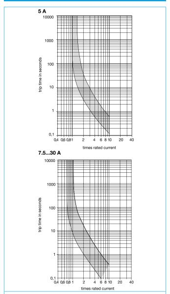
The time/current characteristic curve depends on the ambient temperature prevailing. In order to eliminate nuisance tripping, please multiply the circuit breaker current ratings by the derating factor shown below. See also section Technical information.
