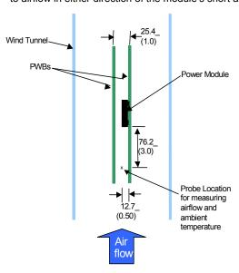
Figure 29. Thermal Test Setup.
