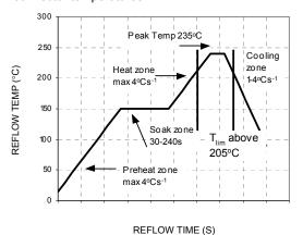
Figure 32. Reflow Profile for Tin/Lead (Sn/Pb) process.
