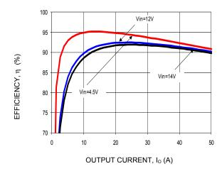
Figure 13. Converter Efficiency versus Output Current.
