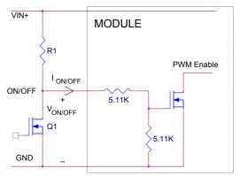
Figure 24. Remote On/Off Implementation using ON/OFF.
