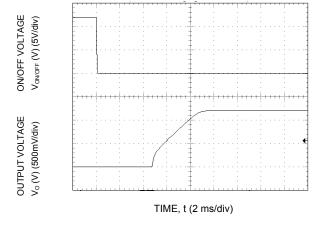
Figure 11. Typical Start-up Using On/Off Voltage (Io = lo,max).
