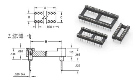
Description: DIP Dual In Line Socket Standard Solder Tail Open Frame Through Hole Plating Code: Shell Plating: 10 μ" Gold over 100 μ" Nickel Inner Contact Plating: 30 μ" Gold over 50 μ" Nickel Packaging: Packaged in Tubes
