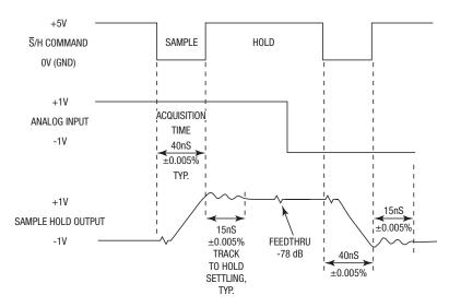
Figure 3. Timing Diagram
