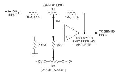
Figure 2. Offset and Gain Adjustments
