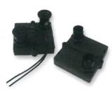
The BDS300 has been designed for use as a snubber resistor where compensatation is required for C-R peaks in traction power supply equipment. The High alumina metallized ceramic is ideally suited to allowing maximum connection to the main heatsink. The resin filled epoxy casing provides large creep distance to mass, large air distance between the terminals and high insulation resistance, whilst the design of the Resitive element element allows for perfect current yeild over the entire component.
