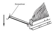
Insert a flat-blade screw driver into the gap under the flaps on the back of the unit as shown in the diagram. Push the screw driver in the direction of the arrow (down).
