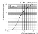
Trigger LED forward current vs.
