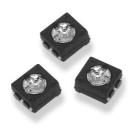
The latest miniaturised sealed trimmer from Citec is the smallest, lightest sealed potentiometer available and the most cost effective. Consuming just 10.5mm² of board real estate, it has been developed specifically for new generation hand held equipment, where double sided component placement is often unavoidable. These 3mm devices are only 1.8mm high. Due to the innovative carbon on polymer technology, the device sets new standards in low cost high reliability electro mechanical components.
