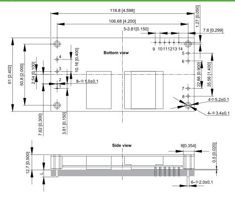
Unit: mm[inch] Bottom view: pin on upside Tolerance: X.Xmm±0.5mm[X.X in.±0.02in.] X.XXmm±0.25mm[X.XX in.±0.01in.]
