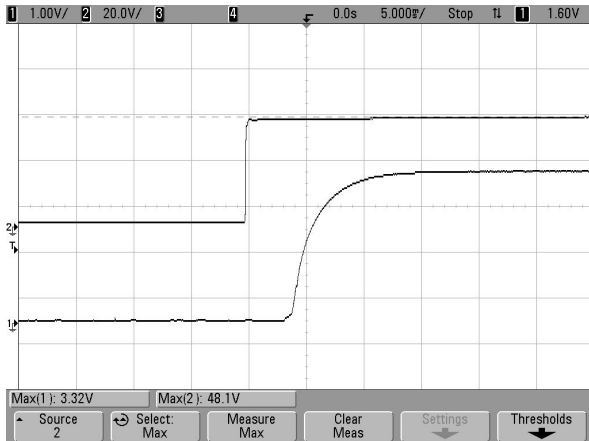
Figure 3 Typical start-up from power on
