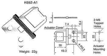
\* After installing the actuator, remove the actuator cover.
