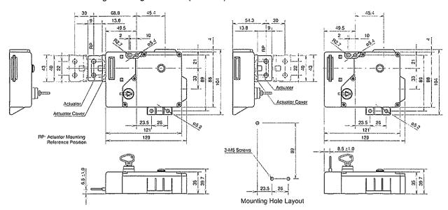
• HS1E with indicator – using the L-shaped actuator (HS9Z-A2)
