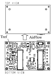
Figure 1. Tref Temperature Measurement Location
