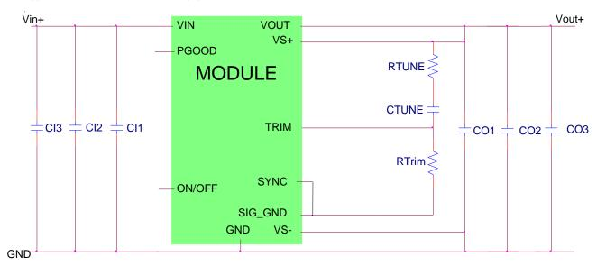
CII Decoupling caps -  $1 \times 0.047 \mu F/16 \text{V}$  ceramic(e.g. Murata LLL185R71C473MA01) +  $1 \times 0.1 \mu F/16 \text{V}$  0402 ceramic
