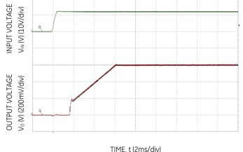
Figure 5. Typical Start-up Using On/Off Voltage ( $I_0 = I_{0,max}$ ).
