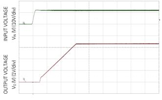
Figure 29. Typical Start-up Using On/Off Voltage ( $I_0 = I_{0,max}$ ).
