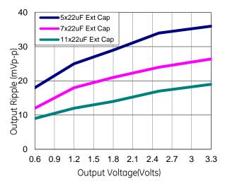
Figure 32. Output ripple voltage for various output voltages with external 5x22 µF, 7x22 µF or 11x22 µF ceramic capacitors at the output (20A load). Input voltage is 12V.
