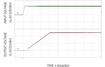
Figure 23. Typical Start-up Using On/Off Voltage ( $I_0 = I_{0,max}$ ).
