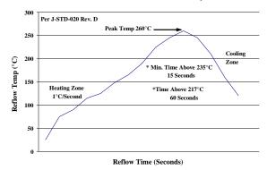
Figure 43. Recommended linear reflow profile using Sn/Ag/Cu solder.
