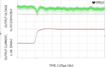
Figure 3. Typical output ripple ( $C_0=7x22\mu F$  ceramic,  $V_{IN}=12V$ ,  $I_0=I_{0,max}$ ,).
