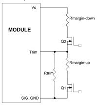
Figure 37. Circuit Configuration for margining Output voltage.
