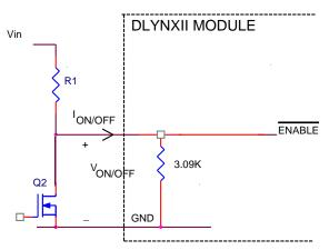
Figure 34. Circuit configuration for using negative On/Off logic.
