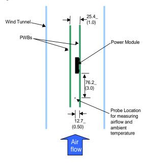
Figure 41. Thermal Test Setup.
