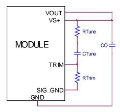
Figure. 40. Circuit diagram showing connection of  $R_{\text{TUME}}$  and  $C_{\text{TUNE}}$  to tune the control loop of the module.
