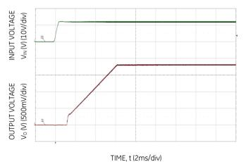
Figure 17. Typical Start-up Using On/Off Voltage ( $I_0 = I_{o,max}$ ).
