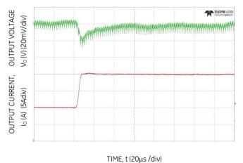
Figure 9. Typical output ripple ( $C_0=7x22\mu F$  ceramic,  $V_{IN}=12V$ ,  $I_0=I_{0.max}$ .).
