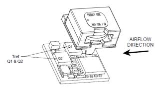
Figure 42. Preferred airflow direction and location of hotspot of the module (Tref).
