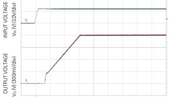
Figure 11. Typical Start-up Using On/Off Voltage (Io = Io, max).
