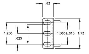
• A CM14 bracket kit consists of two CM5 brackets for the front of the slide and two CM14 brackets for adjustable mounting at the rear of the slide.
