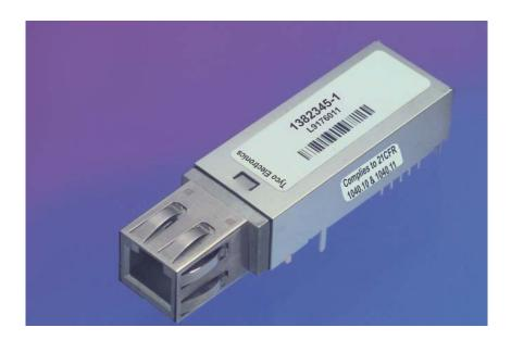
Tyco Electronics' ESCON/SBCON SFF MT-RJ Transceiver 1382345-1 is an LED based 1300 nm fiberoptic transceiver module intended for use in ESCON and SBCON applications. The transceiver sends and receives pre-encoded data over a pair of 62.5 µm or 50 µm core multimode optical fibers. The module, which operates from a single +3.3V power supply, contains separate transmitter and receiver sections with PECL and LVPECL compatible data interfaces.
