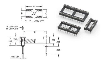
**Description:** DIP Dual In Line Socket Standard Solder Tail Open Frame Through Hole Plating Code: 43
