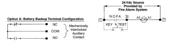
To connect the battery lowering for hydraulic elevator, connect to Points NC and COM.
