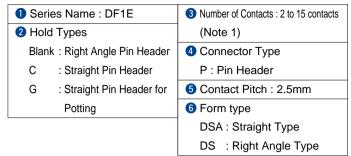
Note 1: Straight pin header for potting has 2 to 11 contacts.
