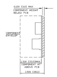
MECHANICAL OUTLINE DIMENSIONS ALL DIMENSION ARE IN INCHES[MM] GENERAL TOLERANCE: ±0.02[0.5mm]
