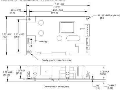
Note: Recommended standoff size is .375" high and all mounting hardware should be less than .28" in diameter. A standoff less than .375" high is acceptable when a thin insulator, 0.4mm thick (polyester, fish paper or equivalent UL rated 94V-2 minimum) is placed between the XL160 and the mounting chassis (refer to applicable UL standard for clearance requirements).
