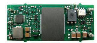
The IBC04-36S12 is the latest wide-range input isolated DC-DC converter specifically designed to supply non-isolated converter architectures. It operates from an ultra-wide input range of 18 Vdc to 60 Vdc and provides a regulated output voltage of 12 V. The output is rated to a power level up to 50 W.
