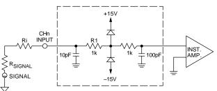
Figure 3. Multiplexer Equivalent Circuit
