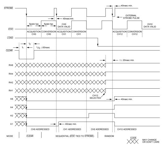
Figure 4. HDAS Timing Diagram
