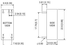
NOTE: Pin tolerance ±0.05mm
