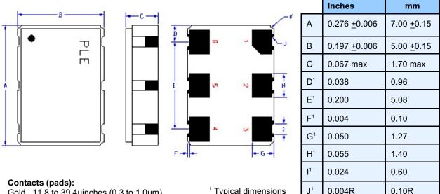
Gold 11.8 to 39.4µinches (0.3 to 1.0µm) over Nickel 50 to 350 µinches (1.27 to 8.89 µm)
