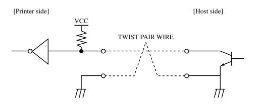
All the output signals are pulled up by 50K
